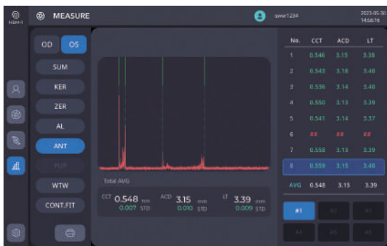
CCT, ACD, LT Measurement
